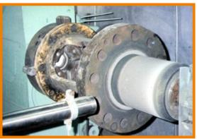
Components in this industry are subjected and exposed to sever wear, heat & corrosion. Many parts are coated with Thermal spray coating to act as excellent high hardness & high toughness barrier to these conditions. Primarily piston rods, shafts & sleeves when worn out by a few hundred microns will lose its applicability in this industry.
