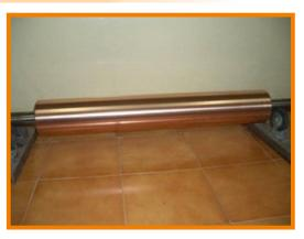
Today's machinery used in Paper & print Industry process very high speed production. The rollers used in the machinery are subjected to severe wear & corrosion by ink and other particles. The gripping of paper is subjected to severe wear and the gripper looses it gripness, hence high strength coatings are required to withstand erosive wear but maintain roughness. Other rollers require low coefficient of friction and to prevent wet paper, adhesives, ink from sticking to rolls surface.
